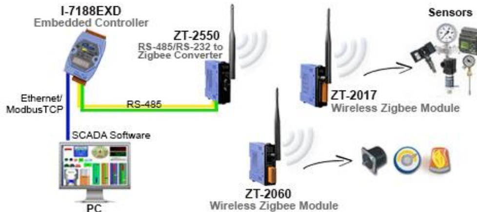
The three topologies defined in the IEEE 802.15.4 are standard, Star, Cluster Tree and Mesh. There are three different types of ZigBee devices in a ZigBee network: coordinator, repeater and slave converter which includes our Zigbee IO modules which have built in IO to save even more wiring costs.
