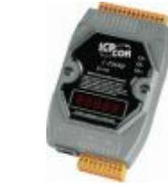
**I-7243D: DeviceNet Master / Modbus TCP Server Gateway** is a solution that provides a communication protocol transfers the DeviceNet and Modbus/TCP to Ethernet.
