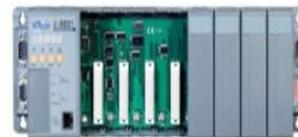
**Modbus TCP and Modbus RTU I/O Expansion Solutions** . Modbus TCP and RTU expansion racks for use with I-87K I/O modules allow you to put more I/O into existing industrial control infrastructures.
