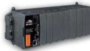
**WP-8841: WinPAC-8000 Controller with 8 slots** VCEP can synchronize every movements (screen, keyboard and mouse actions) between the PC and the WinPAC via Ethernet.
