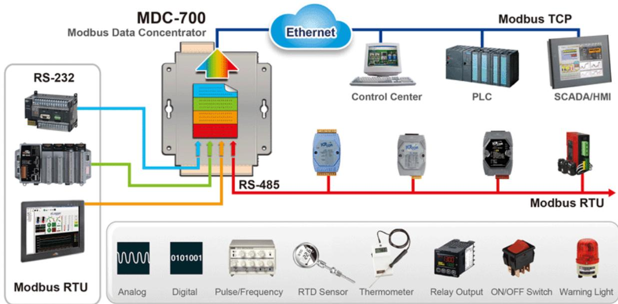
Our solution for this is to add in a **Modbus Data Concentrators (MDC)** for each group of machines or location. Modbus is the most common Industrial protocol and most PLC, Controllers, and industrial software can communicate via this protocol. These MDC improve the efficiency of the SCADA computer by significantly reducing number of devices that are polled and makes data collection more efficient.
