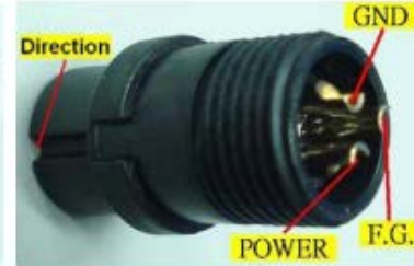
Power Plug Wiring
