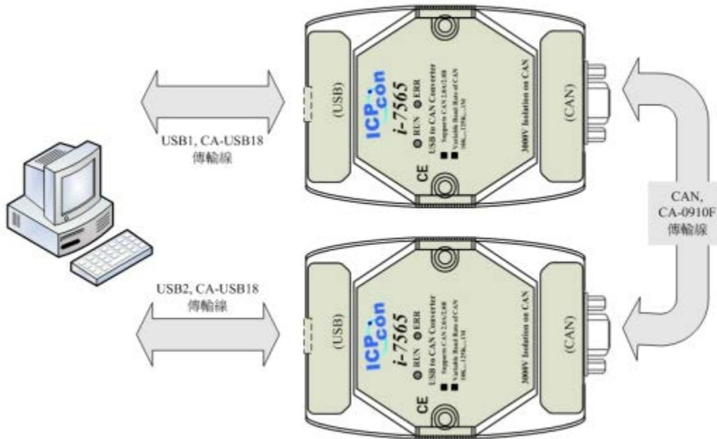
When the I-7565 receives a valid message with the ASCII strings format, it converts this message into a CAN message and transmits it into the CAN network. Based on the same reasoning, when a CAN message is received via the I-7565, the message will be transferred to a message by using the ASCII strings format through the USB port.
