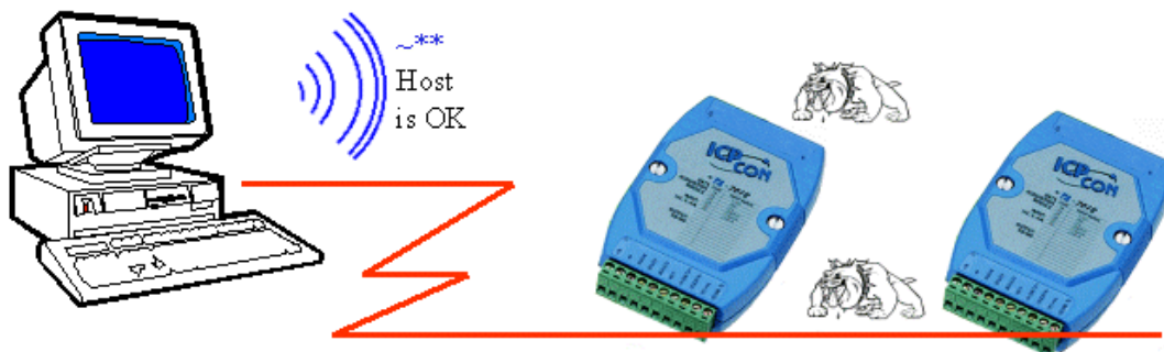
Figure 1. Host PC send command “~**” to every module to notify that the Host PC is OK.
