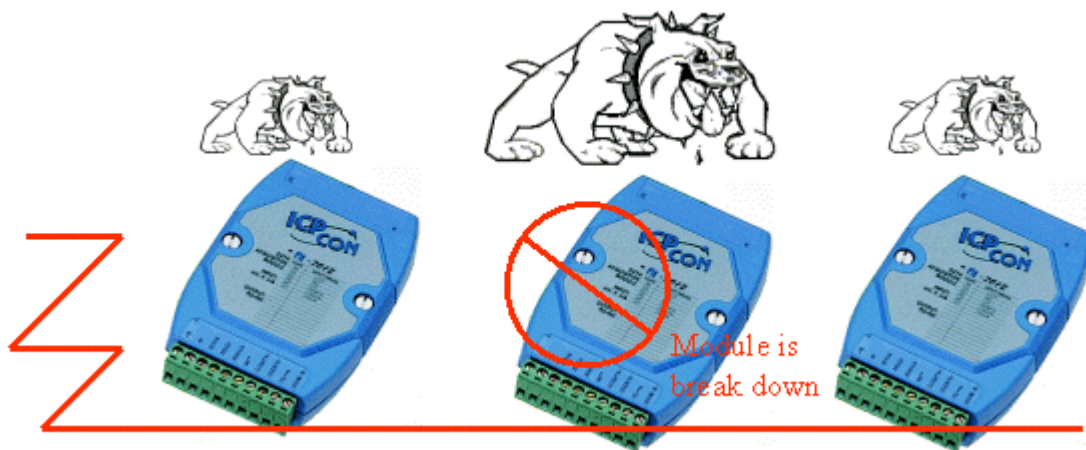
Figure 5. Module Watchdog will reset the module when the module is hanged.
